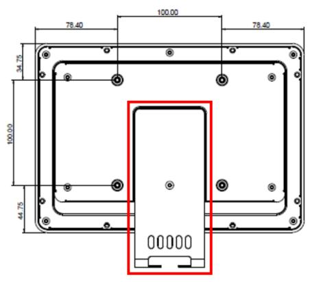
It has five cable slots and a central opening below, centered. The bracket, attached by a single screw, can be removed if desired to facilitate cable connections, then reattached. The slots can hold smaller diameter cables; larger diameter cables can be nested within the confinement area.
